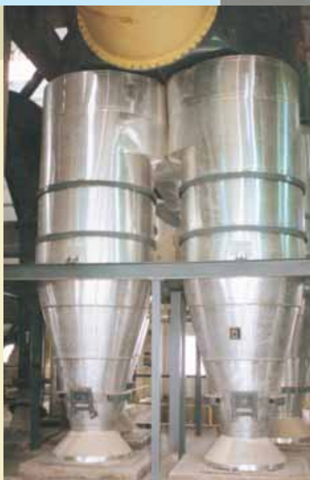
Insulated Quad Cyclones for cooler application in a fertiliser plant
